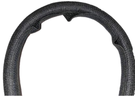
Not OK – Exposed edge on inside of bend
