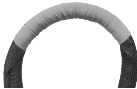
Continuous tape at tight bend
